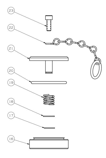
Figure 2 – Exploded Cap Assembly
