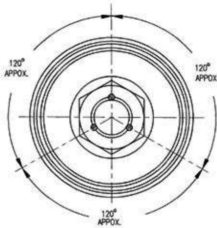
AFTER TORQUING THE SEAT RETAINER NUT, STAKE 3 (THREE) PLACES AS SHOWN ABOVE TO DEFORM THE NUT AND STUD THREADS
