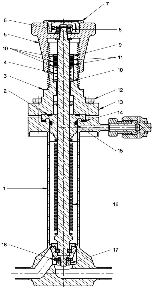
**Figure 1 – Standard Manual Valve**
