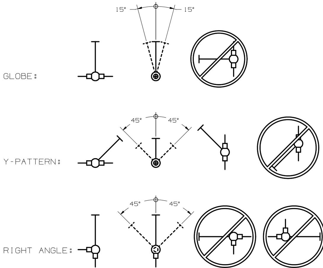
**Figure 4 - Valve Mounting Orientations**
